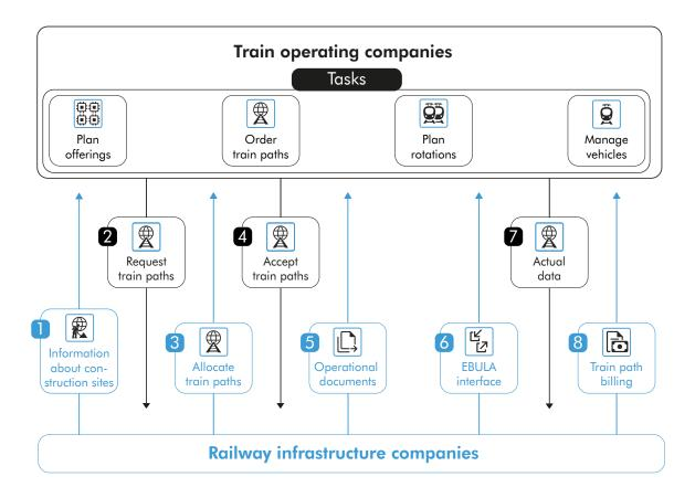
RailSys® offers the capability to plan your timetable, including scheduling, through a web-based platform. With its timetable visualization and scheduling tools, RailSys® provides the necessary instruments for this purpose. These visualizations can be generated for individual days or periods and form the basis for a plausible train path request regarding operational days.
